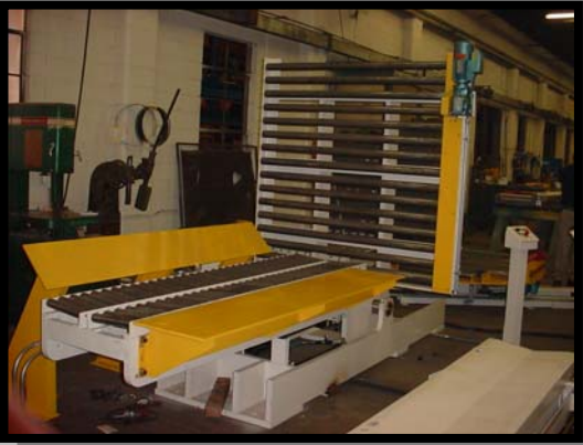
Gravity roller in-feed with a powered roller out-feed
